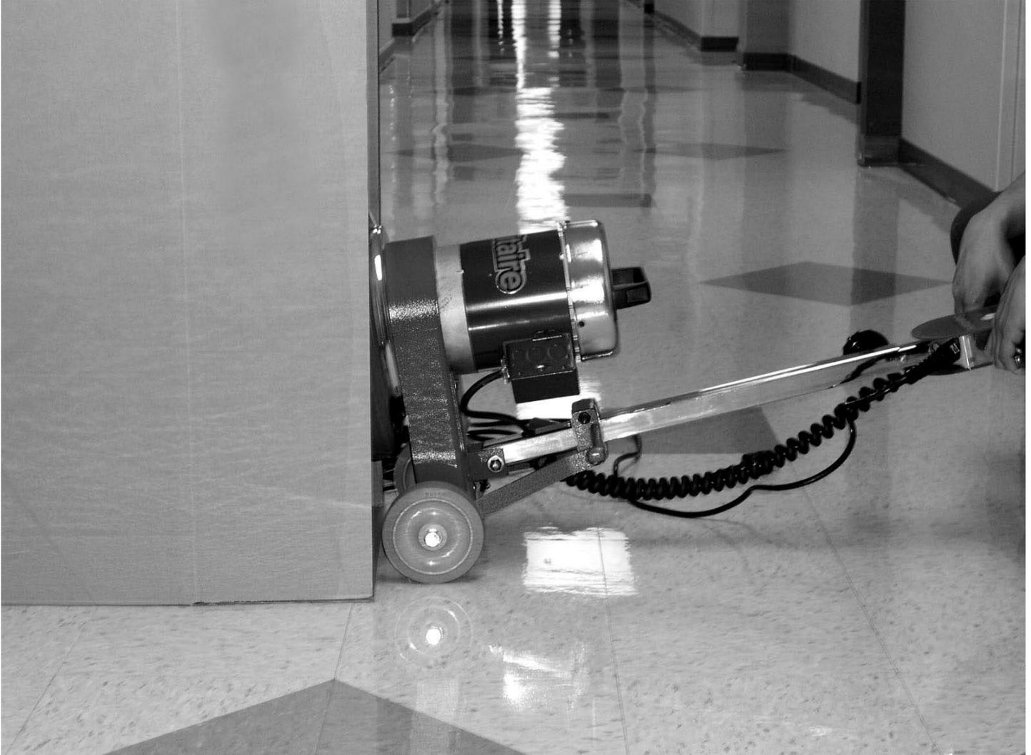
Tip the side of the carton where the wheels are located on its side and roll the machine out of the carton. Loosen the knob on the handle and extend handle to desired height. Tighten knob to secure.
